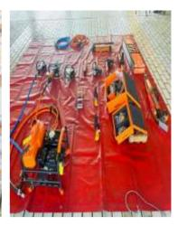
These tools are standard equipment in the firefighter's arsenal of equipment, and they are used to assist vehicle extrication of crash victims, as well as other rescues from small spaces.
