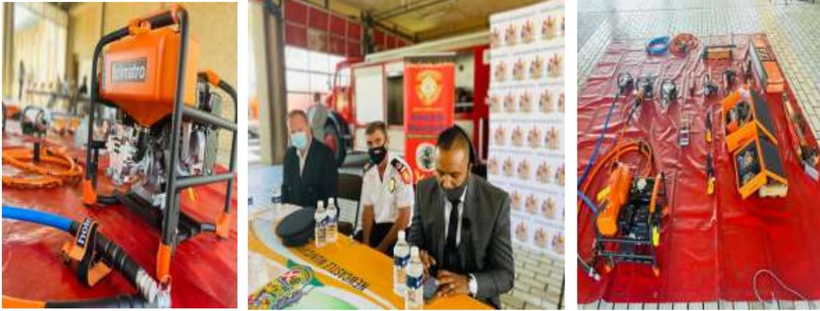
These tools are standard equipment in the firefighter's arsenal of equipment, and they are used to assist vehicle extrication of crash victims, as well as other rescues from small spaces.
