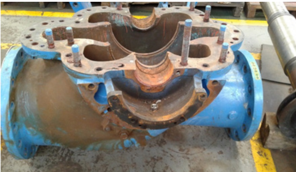
Reconditioning a Split-casing pump at Ngagane Water Purification Plant
