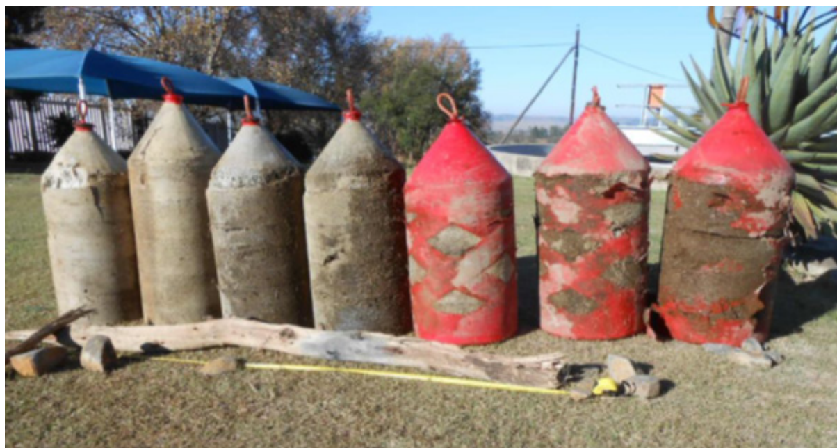
Pigs and recovered Debris after the cleaning operation
