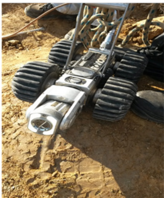
Mobile camera survey of the Tayside pipeline to establish the integrity and condition of the raw water pipeline
