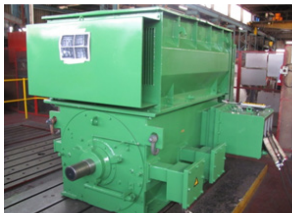
Reconditioned Tayside High Lift Electrical Motor on the Test Bay. Key assets were reconditioned to ensure that their design performance and functionality is restored.
